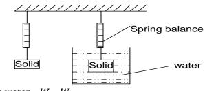
▶ Up thrust in water =  $W_a - W_w$
