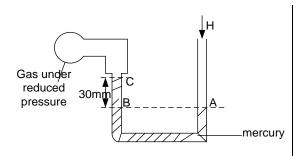
Pressure at B = pressure at A =760mmHg Pressure at C = (H-h) Pressure at C = 760 - 30 = 730mmHgGas pressure = 730mmHg
