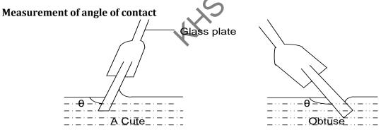
A clean glass plate is placed at varying angles to a liquid until the surface on one side of the plate remains horizontal. The angle  $\theta$  made between the horizontal surface and the plate is the angle of contact.
