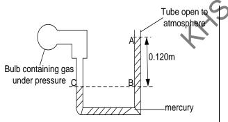
Solution Pressure at C = pressure at B Pressure at C =  $H + h\rho g$ =1.01x10<sup>5</sup>+(0.12x1.36x10<sup>4</sup>x9.81) Pressure of gas = 1.17x10<sup>5</sup>Pa
