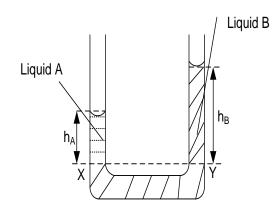
The pressure  $P_x$  at X is equal to atmospheric pressure H plus the pressure exerted by the height  $h_A$  of liquid A i.e.
