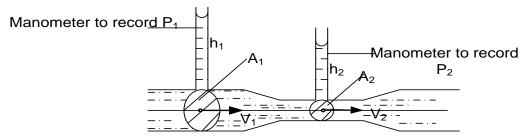
Consider the fluid to be non viscous, incompressible and of density  $\rho$  in a horizontal steady flow let the pressure and velocity be  $P_1$  and  $V_1$  at the main pipe and  $P_2$  and  $V_2$  at the constricted pipe along the same stream line
