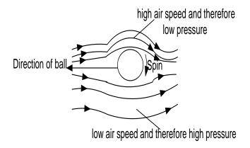
A ball such as a football, tennis or golf ball that is projected to travel through air experiences a sideways force which makes it curve in flight. This is because the spin drags air around with the ball such that air moves faster on one side of the ball than the other. The pressure difference causes a resultant force which makes the ball the curve as it spins.
