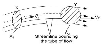
In a time interval  $\Delta t$  the fluid at X will move forward a distance  $V_1\Delta t$ . therefore, a volume  $A_1V_1\Delta t$  will enter the tube at X. the mass of fluid entering at X in time  $\Delta t$  will be there be
