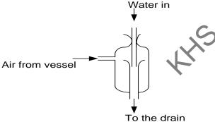
This pump has a narrow cross section in the middle so that the jet of water from the top flows faster here. This reduces the pressure around it and thus air flows in from the side of a tube connected to a vessel. The air and water are expelled together through the bottom of the pump
