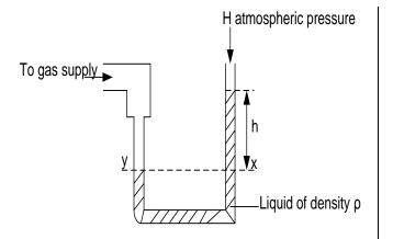
The gas pressure p is the same at the pressure at y But pressure at y = pressure at x  $P = H + h\rho g$ Where  $H = 1.01x10^5 Pa$ Or H=760mmHg Or H=76cmHg
