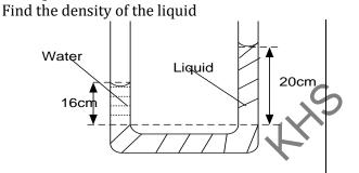
$P_{x} = H + h_{A} \rho_{A} g$ Where  $\rho_{A}$  is the density of liquid A Similarly at Y  $P_{y} = H + h_{B} \rho_{B} g$ Where  $\rho_{B}$  is the density of liquid B Since x and y are at the same level  $P_{x} = P_{y}$   $H + h_{A} \rho_{A} g = H + h_{B} \rho_{B} g$  $\boxed{h_{A} \rho_{A} = h_{B} \rho_{B}}$
