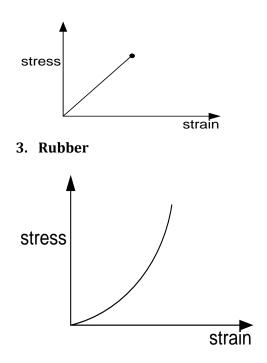
Brittle materials have only a small elastic region and do not under go plastic deformation. This behavior in glass is due to the existence of cracks in its surface. The high concentration of the stress at the crack makes the glass break.
