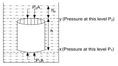
Volume of fluid displaced = volume of cylinder
